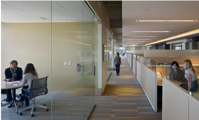
*On the interior of the building, shading devices control glare and minimize heat gain while light shelves facilitate daylight harvesting.*
